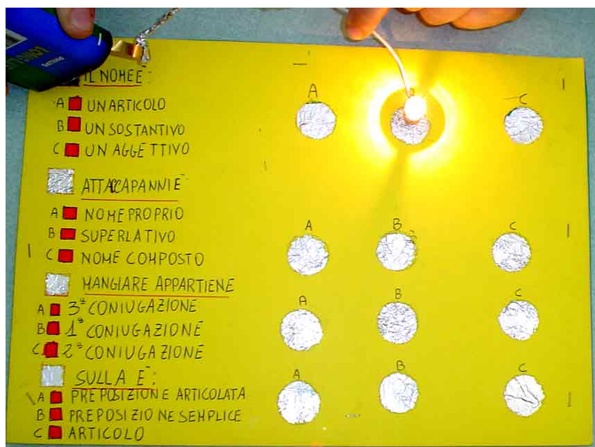
Figure 1. A wire-card quiz made by pupils along with the battery - bulb tester.
