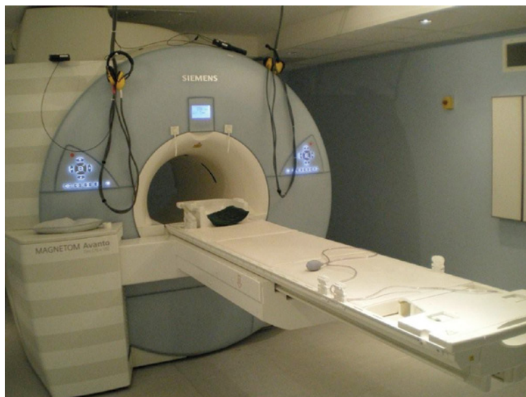
Figure 2.5 A 1.5 T MRI scanner, fitted for research purposes. (Courtesy Birkbeck/UCL Centre for NeuroImaging.)
