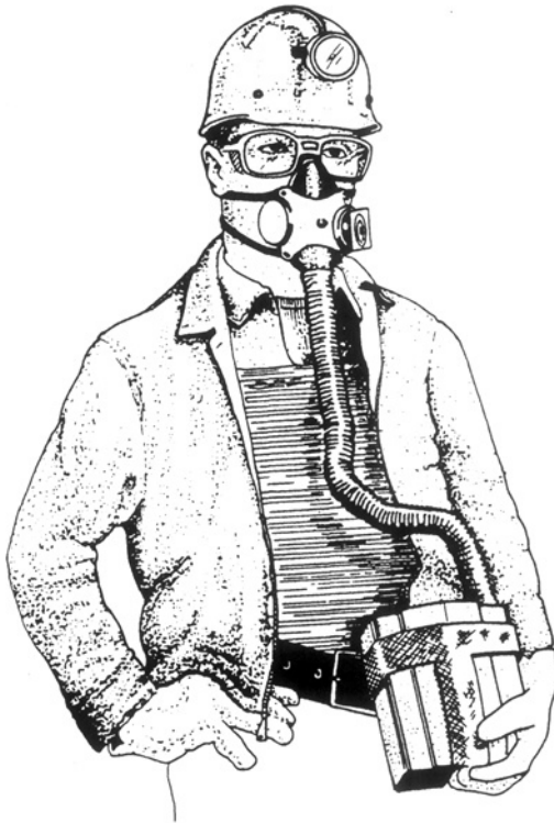
FIGURE 4.16 Positive-pressure respirator (Divers and Cecala, 1990).
