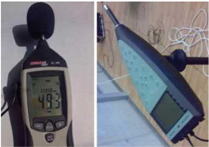
Fig. 5.13 Simple sound-pressure level meters evaluate the sound’s loudness over the whole frequency range (between 20 and 16,000 Hz) and only offer “F” and “S” time averaging (left). Even state-of-the-art meters evaluate the sound-pressure levels only in discrete frequency bands [4] (right)
