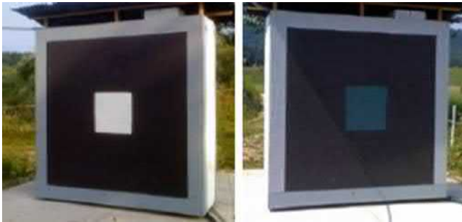
Fig. 1.23 On a sunny day at noon, the temperature of the facade painted with selective paint was up to 13^\circ\text{C} lower comparing to none selective facade; selective white colour layer with high reflectivity of none visible part of solar radiation was laid first and after green shaded layer having a high thermal radiation emissivity \varepsilon_{IR} was added [5]
