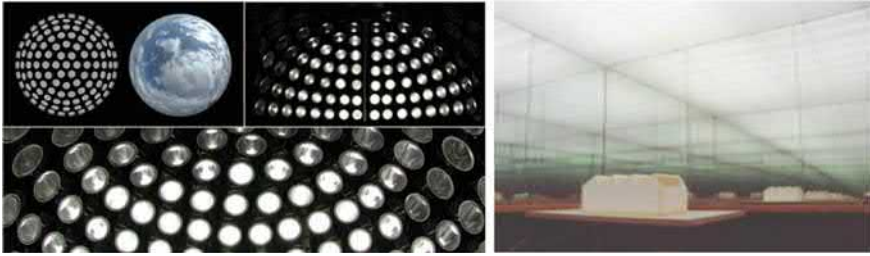
Fig. 4.59 Hemispherical (left) and box-type artificial sky simulator with mirrors (right). A rectangular box with mirrors can be used for daylighting analysis under the conditions of an overcast sky, the hemispherical artificial sky can simulate any sky luminance distribution [26, 27]
