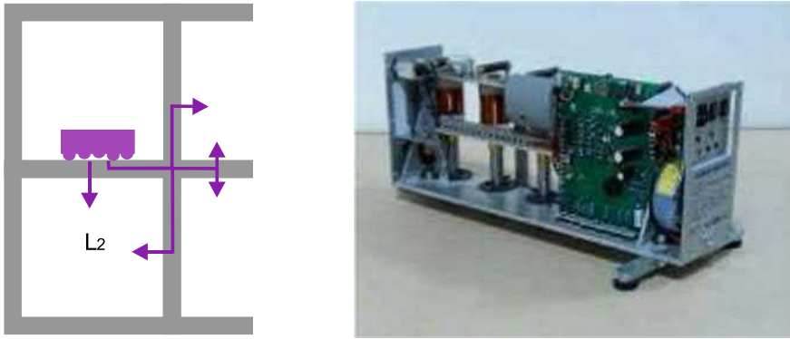
Fig. 5.63 Impact sound is transmitted to adjacent rooms through partition and mezzanine building structures (left). A standardised device for impact sound generation is placed directly on a building structure [27] (right)
