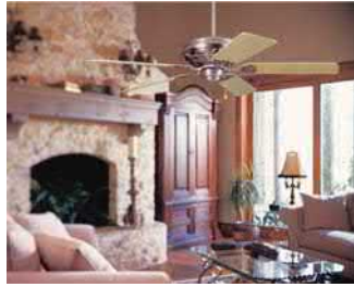
Fig. 1.107 A ceiling fan does not cool the air, but perceived temperature in the room is lower due to the higher air velocity. The perceived temperature for an air velocity 1 m/s next to the skin is 3 °C lower compared to still-air conditions
