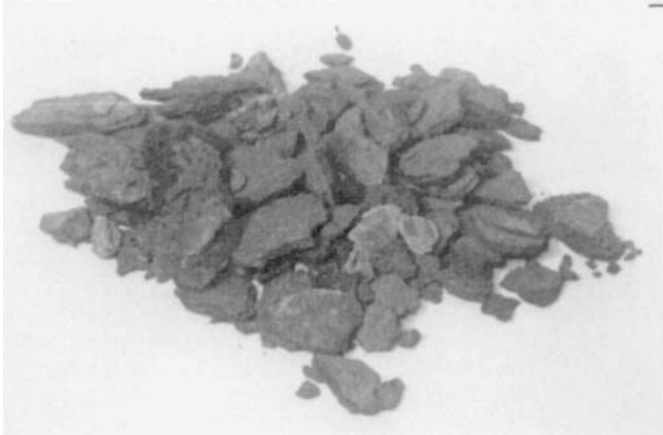
FIGURE 8.5.23 Pipe scale and iron corrosion products. (Courtesy of The Metro Group, Inc.)
