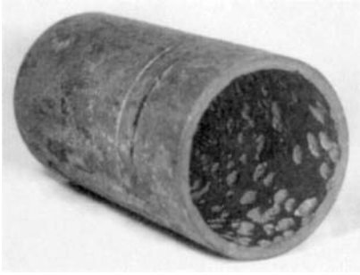
FIGURE 8.5.18 Pitting in boiler feedwater line. (Courtesy of the Metro Group, Inc.)
