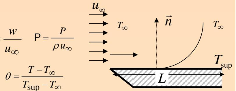
$$\theta = \frac{T - T_\infty}{T_\sup - T_\infty}$$
