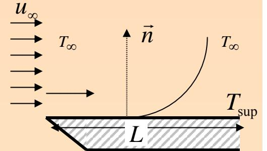
$$\theta = f(Re, Pr, Ec) \quad \theta = \frac{T - T_\infty}{T_{\text{sup}} - T_\infty}$$
